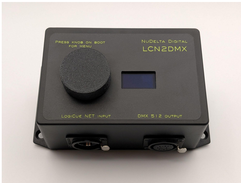
[PHOTO 1: Front of the unit — OLED display and encoder knob]
